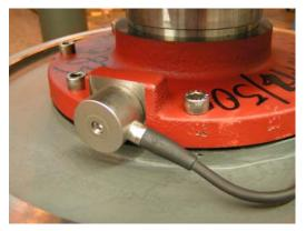
Figure 5-29 Acceleration Sensor on Locating Bearing
