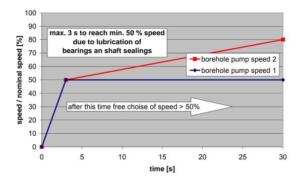
Figure 4-4 Typical Ramp Profile for borehole pump
