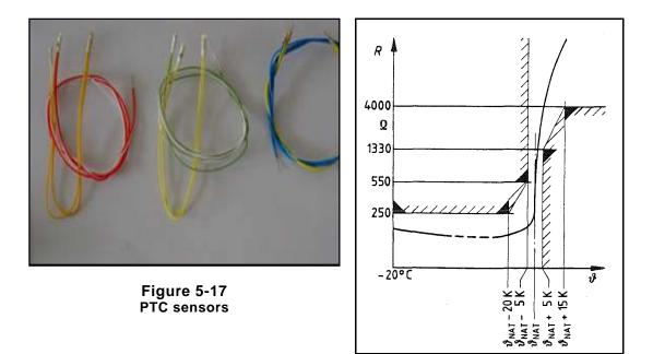
Figure 5-18 PTC characteristic acc. DIN 44082
