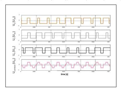
Figure 3-4 Formation of Common Mode Voltage from Phase Voltage Pulses
