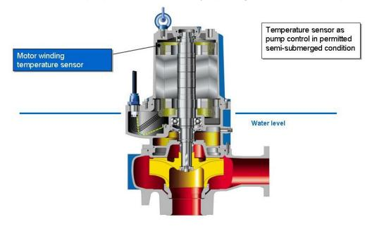
Figure 5-20 Semi Submerged Operation
