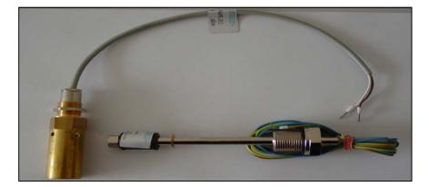
Figure 5-25 Different Types of Float Switches
