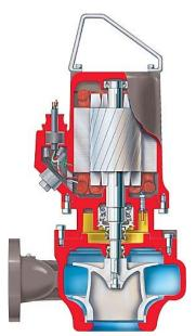
Figure 5-15 Typical Oil Filled Motor Sewage Pump-set
