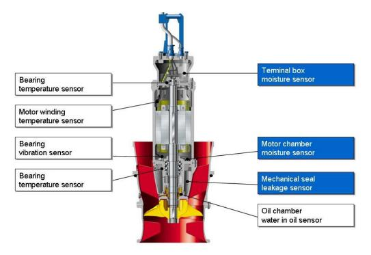
Figure 5-23 Leakage Sensors
