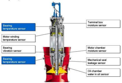
Figure 5-21 Bearing Temperature Sensor
