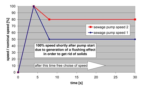
Figure 4-3 Typical Run up time for sewage pump
