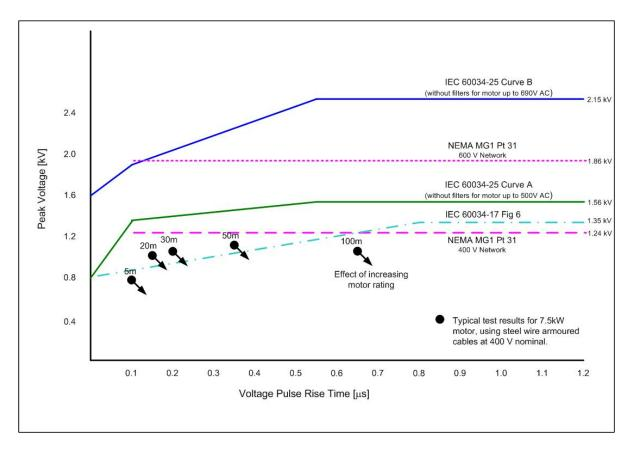
Figure 1-1 Voltage withstand curve
