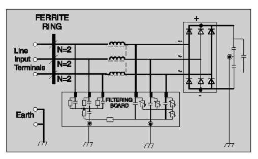
Figure 5-1 Typical Conducted Emissions Filter, Integrated into Drive Module
