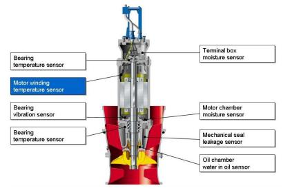
Figure 5-16 Motor Winding Temperature Sensor
