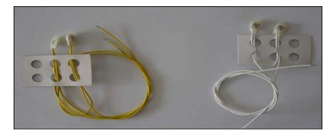
Figure 5-19 Thermal (Bi-metal) Sensors
