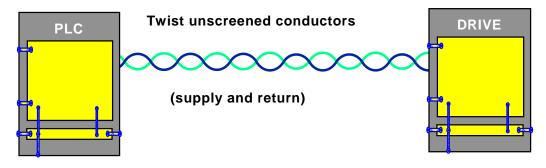
Figure 5-6 Twist all Control Cable Pairs
