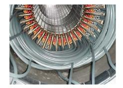
Figure 3-2 Example of Wet Wound Motor Under Construction
