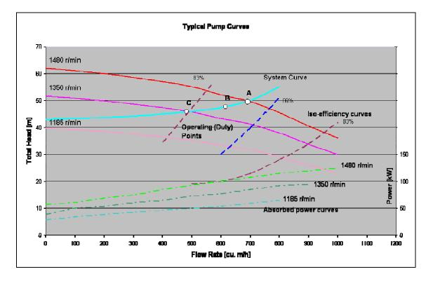
Figure 4-1 Example of the effect of pump speed change with a system with high static head.
