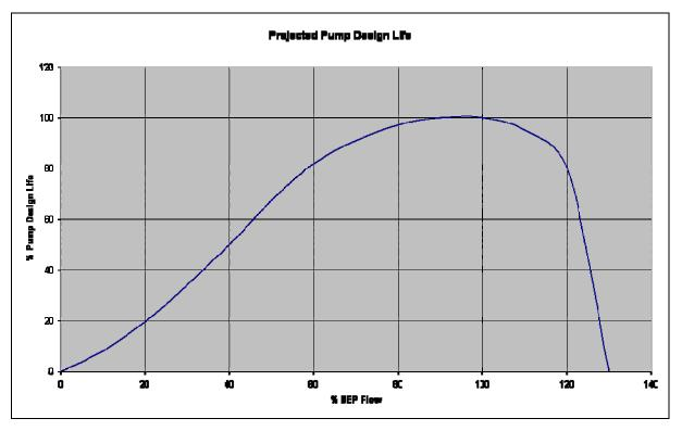
Figure 4-2 Projected %Pump Design Life vs % Flow Rate
