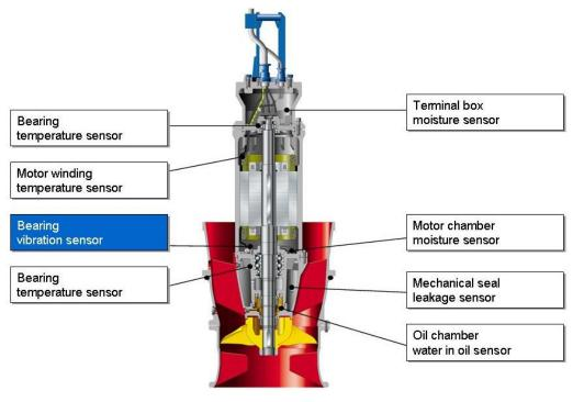
Figure 5-28 Vibration Sensor
