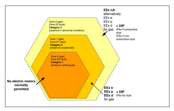
Figure 7-1 Permitted Equipment Categories for different hazard levels
