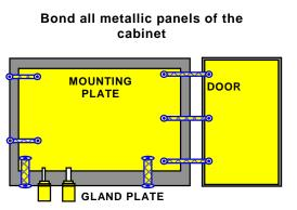
Figure 5-4 Enclosure Grounding Requirements
